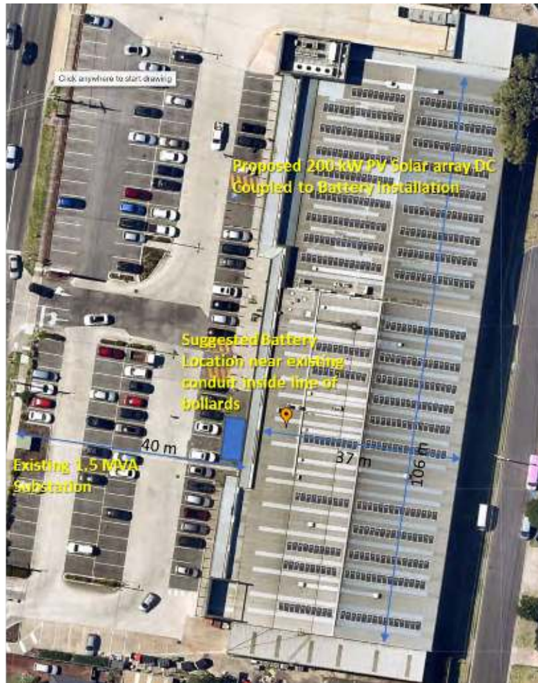
Image 11. Ariel image of North Geelong shopping centre with proposed PV array.
